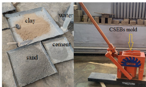
Fig. 2. CSEBs raw materials and molding machine for CSEBs production.
