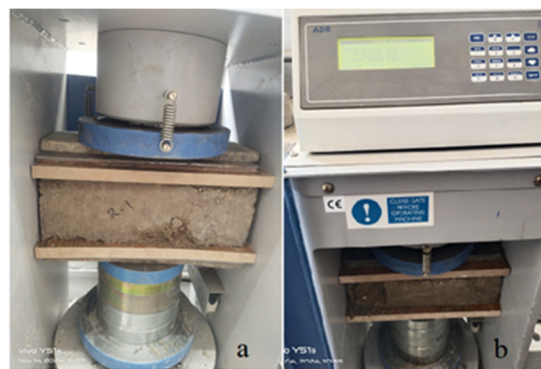
Fig. 3. Illustrates the, a) dry state and b) wet-state compression tests on CSEBs
