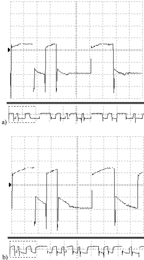
Figure 4. Oscilloscope waveform with matching resistors at 115200 baud speed: a) 75 Ohm matching resistor; b) 195 Ohm matching resistor.
