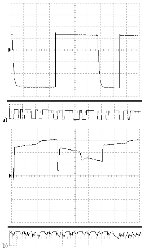
Figure 3. Oscilloscope waveform without matching resistors use: a) 1200 baud speed; b) 115200 baud speed.
