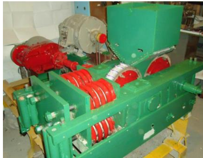
Figure 1. Experimental installation of a press roller machine with a device for directing anisotropic materials
