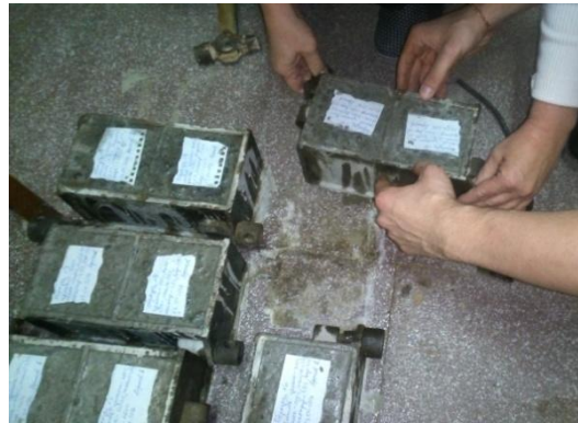
Figure 2. The process of extracting laboratory samples from molds.
