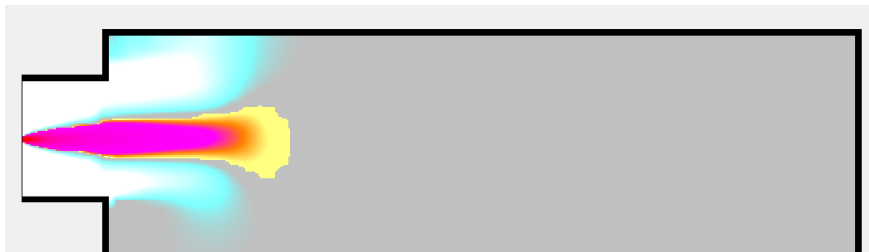
Figure 4. View from above on the diffusion fame in the glass furnace with returned gases flow
