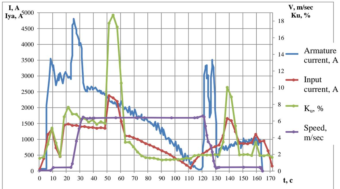
**Figure 2.** A diagram of vehicle speed alteration, armature current and input current, total harmonic components of the voltage over a cage hoist lift cycle.
