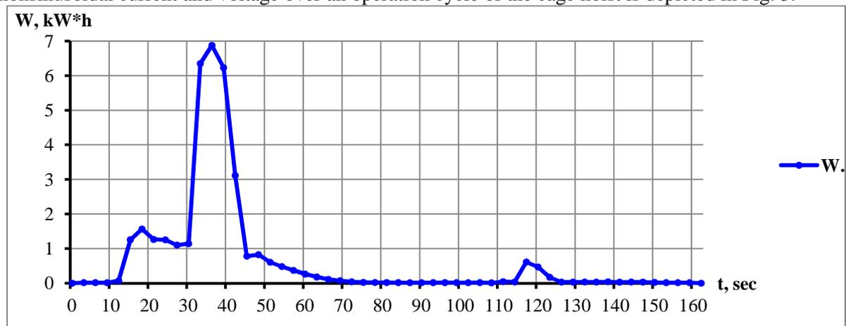
**Figure 3.** The electric energy losses conditioned by nonsinusoidal currents and voltages of the power line over a single hoist operation cycle.
