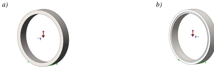
**Figure 3.** Boundary conditions for tyre models: *a)* reference; *b)* reconstructed
