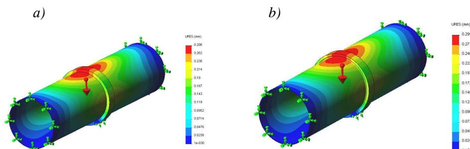
**Figure 11.** Displacement profiles of the studied tyre models: *a)* reference; *b)* reconstructed
