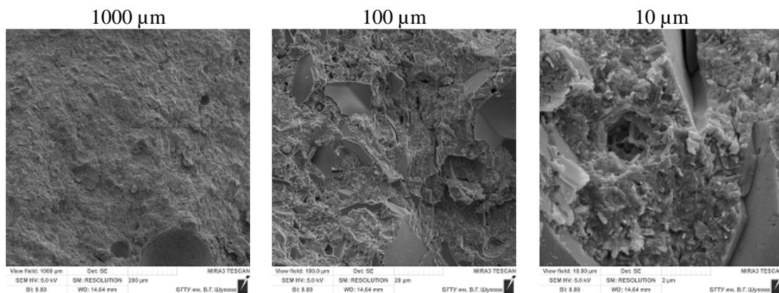
**Figure 8.** Cement stone microstructure from binding composition 15 cured for 28 days
