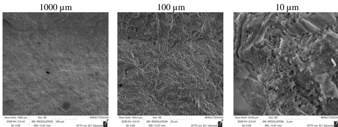
**Figure 6.** Cement stone microstructure from Portland cement activated in vortex jet mill (3 passes) cured for 28 days
