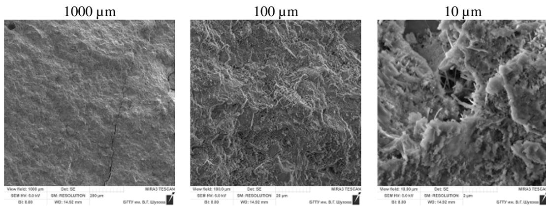
**Figure 4.** Cement stone microstructure from Portland cement activated in vortex jet mill (1 pass) cured for 28 days
