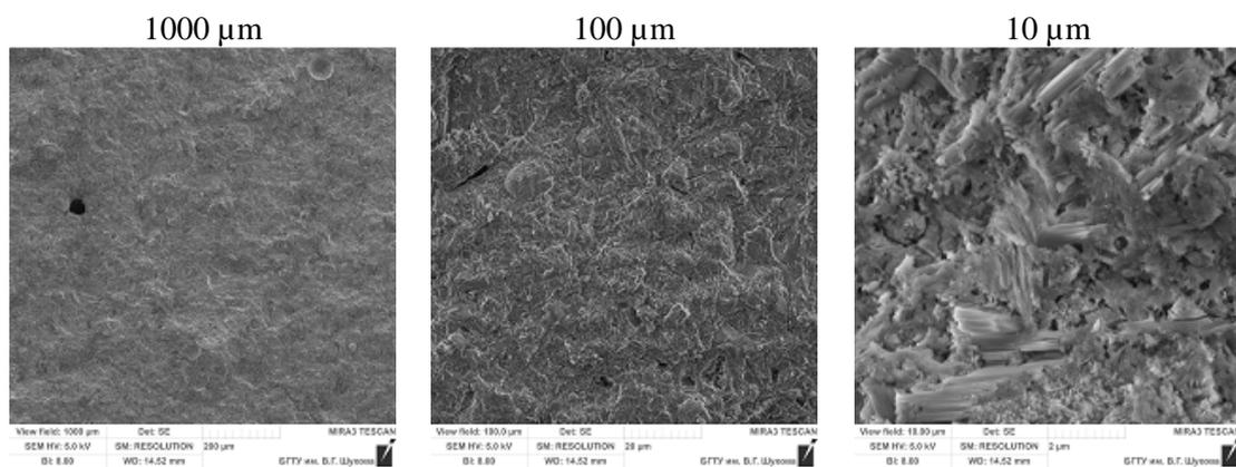
**Figure 5.** Cement stone microstructure from Portland cement activated in vortex jet mill (2 passes) cured for 28 days
