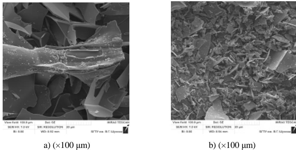
**Figure 1.** Initial perlite waste (a) and perlite waste milled in vortex jet mill (b)
