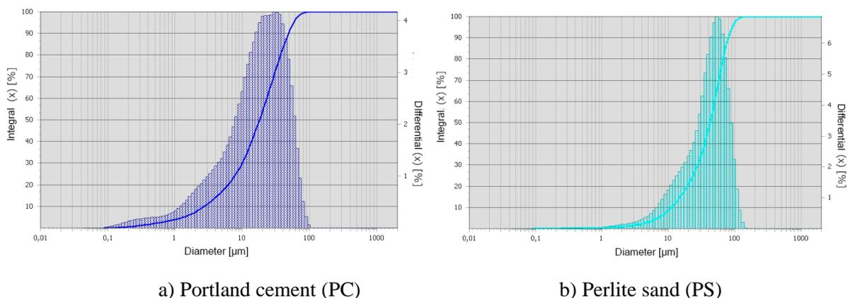
**Figure 2.** Cement particle size distribution (a) and perlite waste particles size distribution (b)
