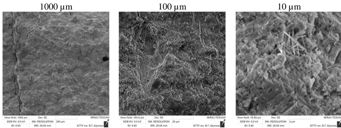
**Figure 3.** Cement stone microstructure cured for 28 days
