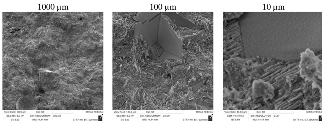
**Figure 7.** Cement stone microstructure from binding composition 6 cured for 28 days
