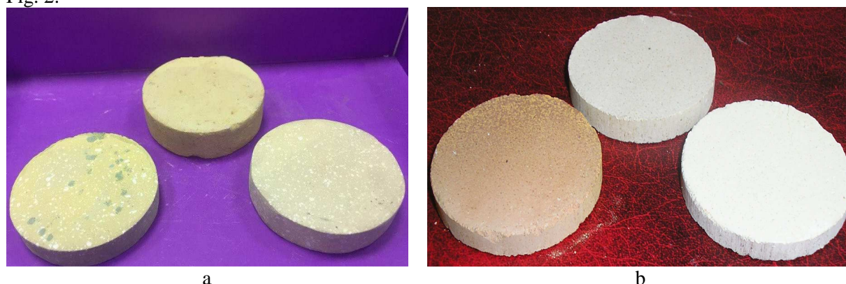
Figure 2. General view of samples after firing: a – on the basis of alumina suspension, b – on the basis of chamotte suspension
