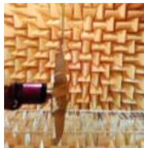
Figure 6. Test for propeller performance of designed propeller was identified. geometry in anechoic chamber
