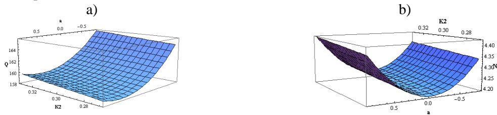
Figure 3. Influence of the angle of inclination of the ES on Q, N, q for different values of the loading of the grinding bodies of the second chamber, ( \varphi_1 = 0.16 ; \xi = 0^\circ ; l_1 = 0.6 )
