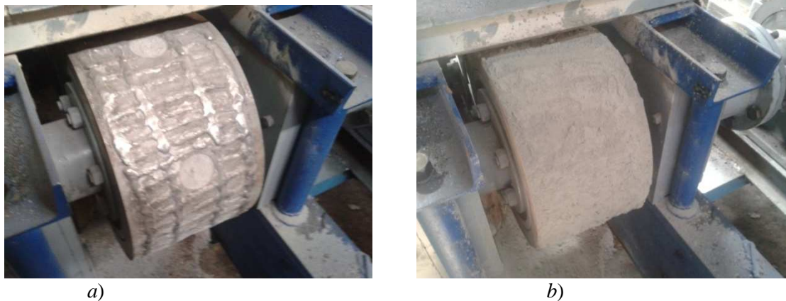
Figure 3. Rolls PRG with welded mesh on their working surface: a - before the grinding process; b - after grinding
