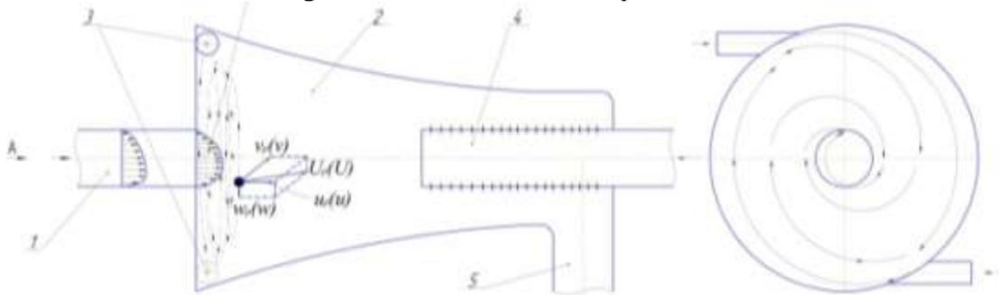
**Figure 1.** A scheme of the vortex motion of a two-phase flow in a homogenization chamber: 1 - transportation of the components of the mixture over the accelerating unit; 2 - homogenization chamber; 3 - tangential air blowing; 4 - unit for aeration and disaggregation of the mixture; 5 - discharge fitting.
