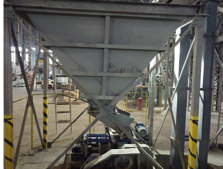
Figure 3. Press roll grinder with deagglomerating device
