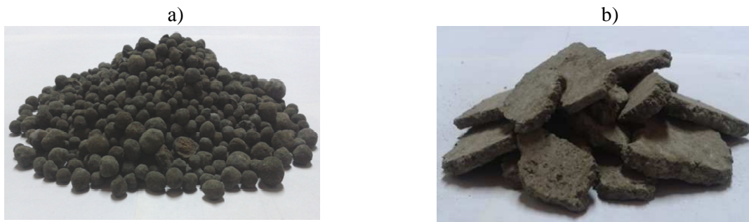
Figure 1. Clinker material to be grinded: a) - initial product; b) - after treatment in PRG
