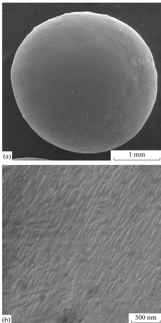
**Fig. 1.** SEM-image of the THP surface microstructure, obtained at (a) 80- and (b) 100000-fold magnification.
