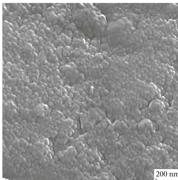
**Fig. 2.** SEM-image of the surface microstructure of a titanium-coated THP (200000-fold magnification).
