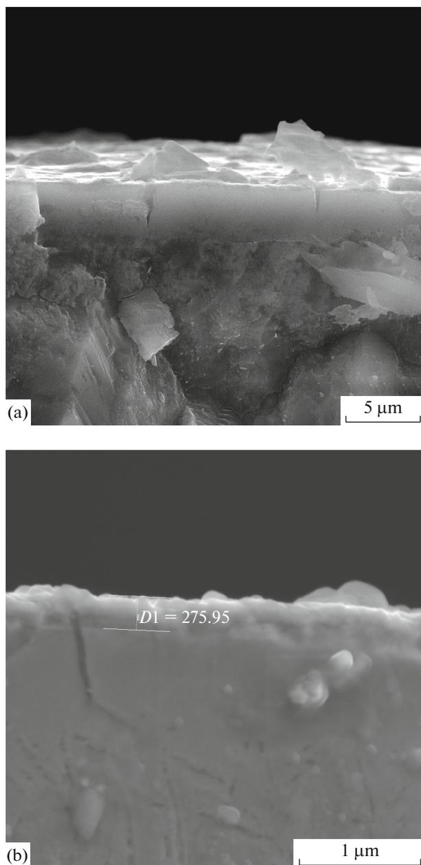
**Fig. 3.** SEM-image of the surface microstructure of a titanium-coated THP at (a) 10000- and (b) 80000-fold magnifications.
