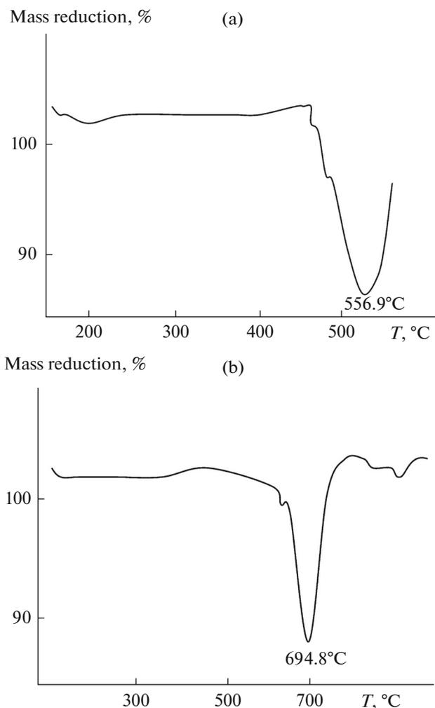
**Fig. 4.** Curves produced as a result of the differential thermal analysis of (a) the initial THP and (b) of the titanium-coated THP.
