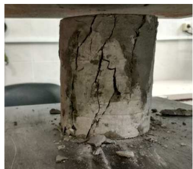
Figure 3. Unsatisfactory fracture pattern in cylindrical samples collected from cast in-situ structures
