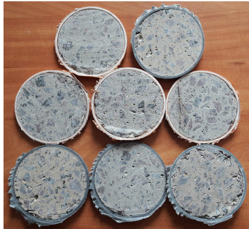
Figure 2. Solid nature of concrete core in tested PTC samples
