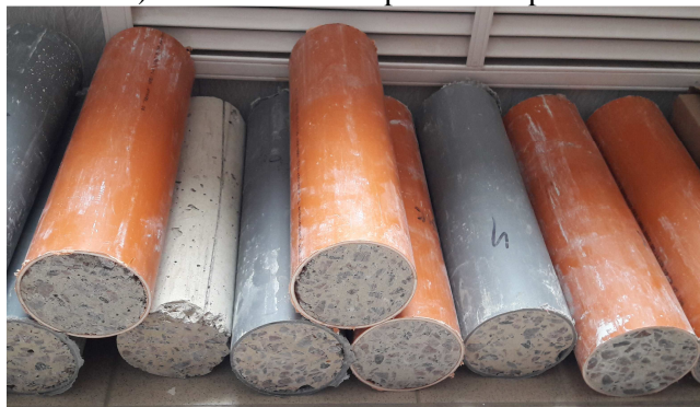
Figure 1. Samples of PTC short columns.
