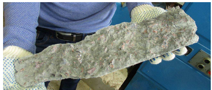
Fig. 3. Monolithic nature of concrete in tested specimens
