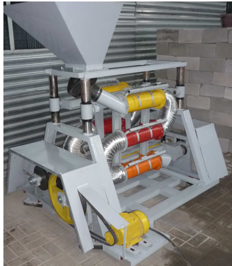
Figure 3. A general view of the centrifugal grinding unit with parallel blocks
