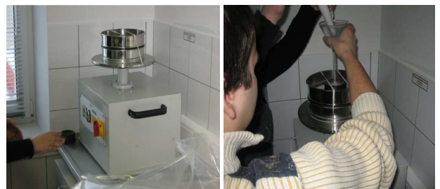
Fig. 1. Method of determining cement flowability by the ASTM 1565-04 method: a) a shaking table Hagerman with sieve number 05 installed on it; b) loading material on sieve number 05
