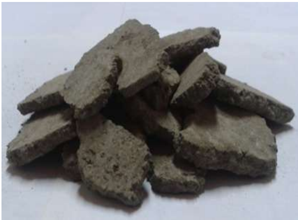
Fig. 2. Clinker's shape after grinding in PRS
