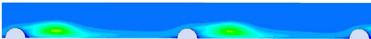
Fig. 4. Graphical allocation of the flow turbulence with different crosscut flow speed for cylinder-formed ribs, with 2 mm height.
